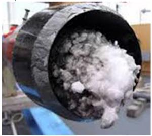
If the temperature of the fluid in the pipeline goes below the hydrate formation temperature, hydrate plug could form in the pipeline leading to blockage and consequently production loss. We adopt two-pronged approach of hydrate management as below:
