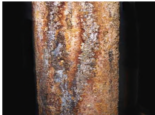
Figure 2 General corrosion of external surface of pipework
